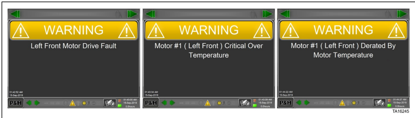
Figure 39. Examples of Yellow Warnings Associated with Motor Over-Temperature
