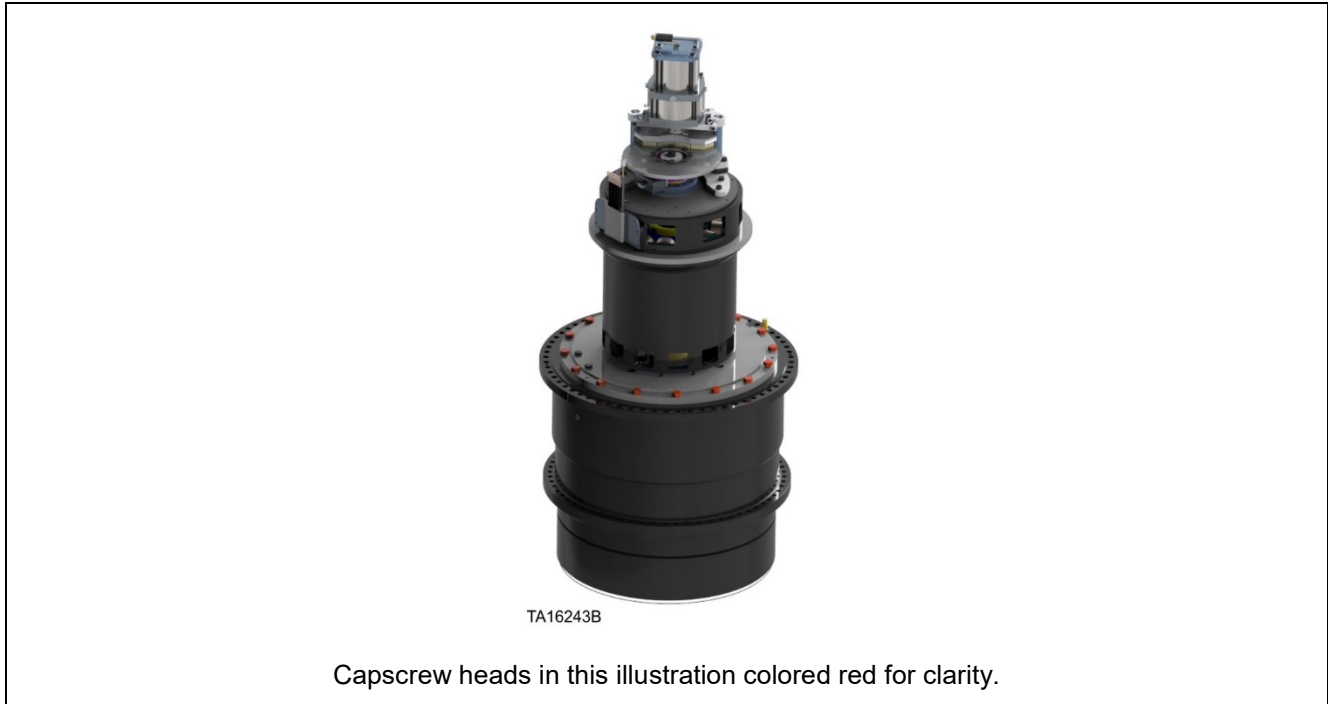
Figure 46. Install all motor-to-planetary drive capscrews
