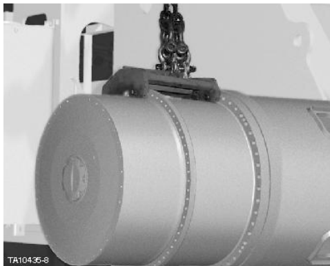
Figure 19. Crane attachment for removal of traction motor/planetary drive/assembly
