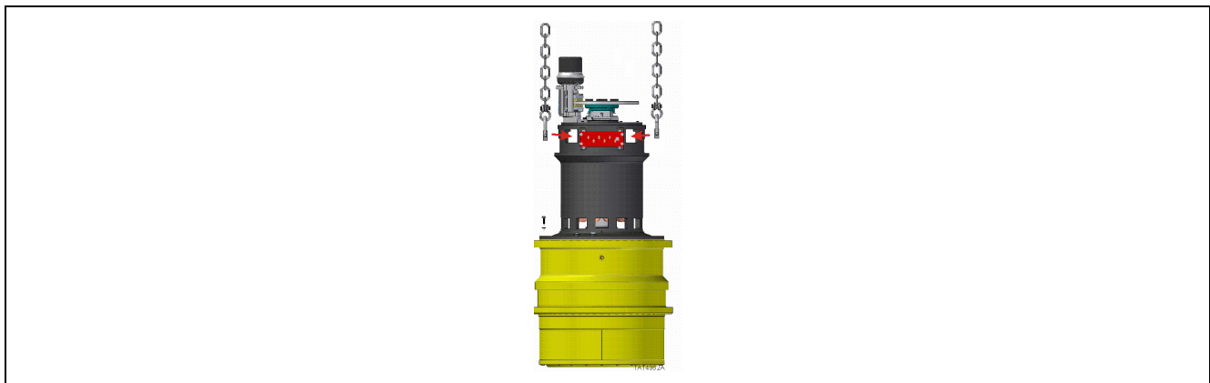
Figure 25. Planetary drive and traction motor positioned for motor removal
